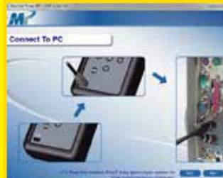
Connect the USB cable supplied to the BRT-12 and then to a USB port on the PC. A main USB port (on the rear of the PC) as opposed to an extension (on the front of the PC) is preferable.
