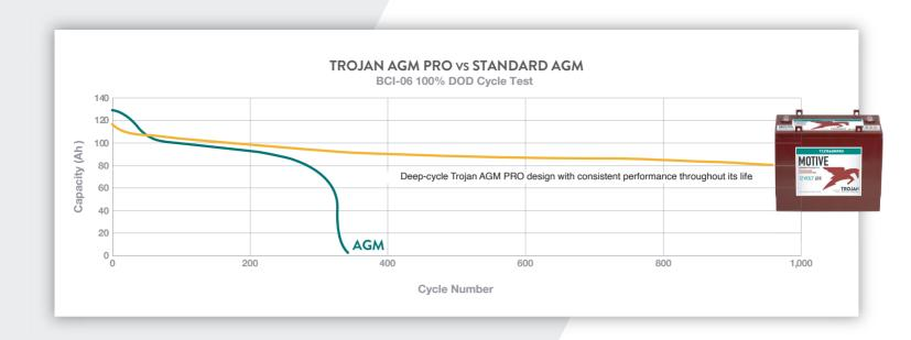
Trojan AGM PRO maintains high capacity in extreme deep-cycling with consistent performance throughout its life compared to standard AGM.
