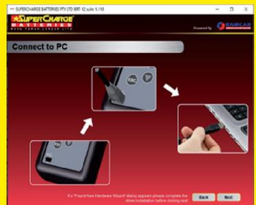
Connect your BRT-12 as per the instructions within the Supercharge Batteries PC suite. Connect mini-USB to Supercharge Batteries BRT-12 and USB to PC. Refer to the 'Updating the Supercharge Batteries BRT-12' section for more information.
