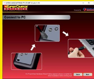
Connect the USB supplied to the BRT-12 and then to a USB port on the PC.
