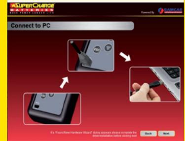
Connect the USB supplied to the BRT-12 and then to a USB port on the PC.
